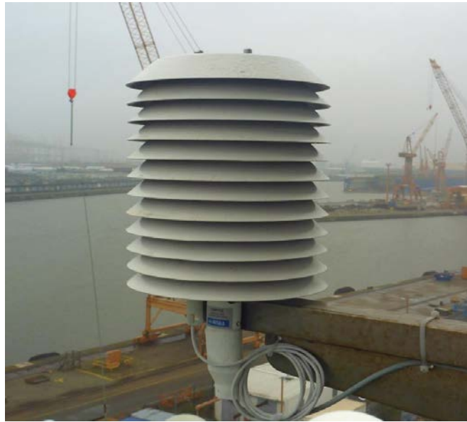
Figure 1. Temperature and humidity sensor (PRT), protected from solar radiation, on board R/V Polarstern. Similar instrument is installed on both sides of the ship. For analyses, data of windward sensor is used.
