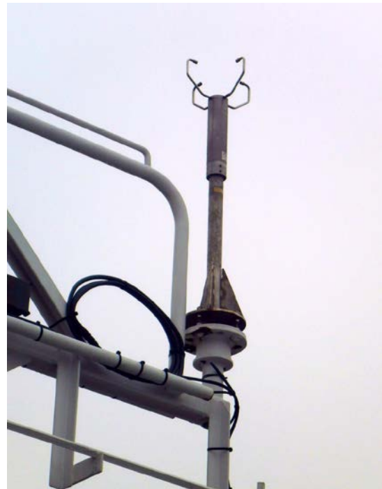
Figure 2. Ultrasonic anemometer on board R/V Polarstern. Similar instrument is installed on both sides of the ship and data is read from the sensor better exposed to wind.
